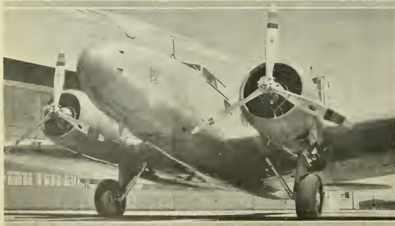
One of the new Boeing 247-Ds with geared Wasps and three-bladed propellers
